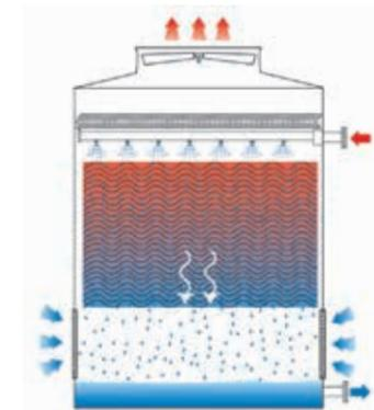
Figure 2: Open circuit cooling tower
