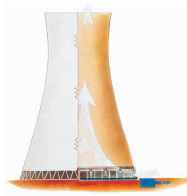
Figure 9: Natural draft cooling tower
