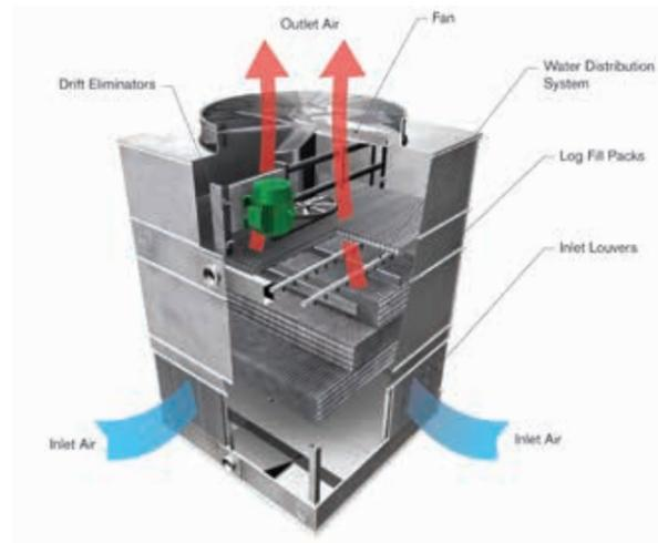
Figure 5: Counter flow cooling tower
