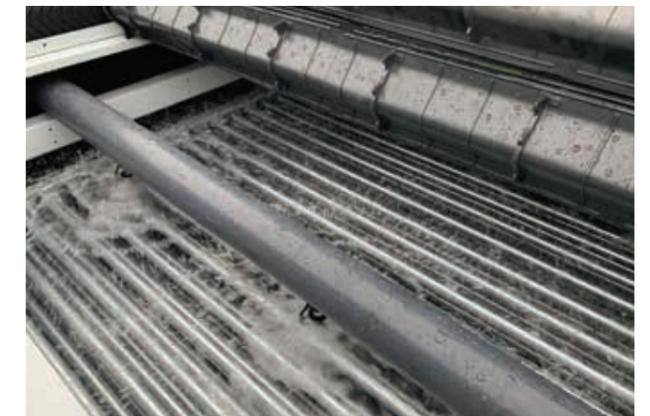
Figure 22: Pressurised spray water distribution
