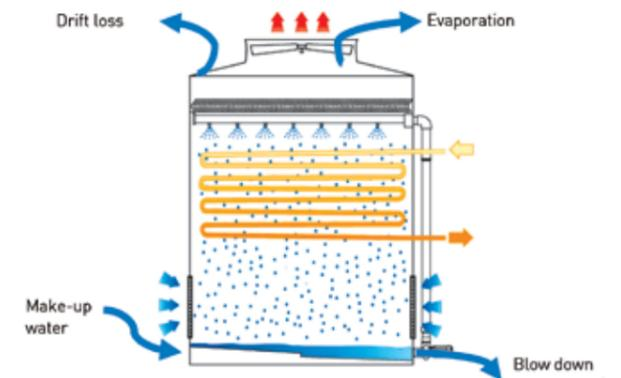
Figure 3: Closed circuit cooling tower
