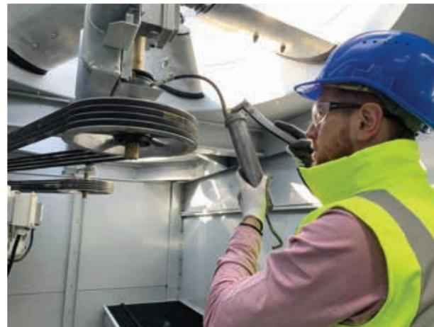
Figure 27: Greasing the bearing
