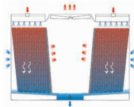
Figure 7: Induced draft, cross flow cooling tower
