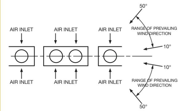
Figure 14: Installation relative to prevailing wind direction
