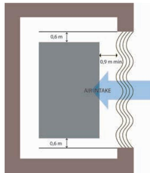
Figure 18: Louvered wall enclosure
