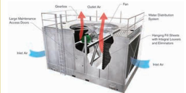
Figure 4: Cross flow cooling tower
