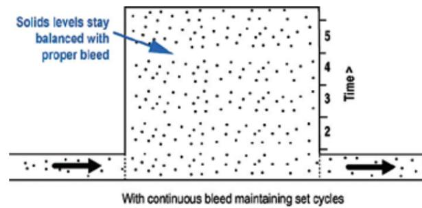
Figure 26: Continuous blow down cycles
