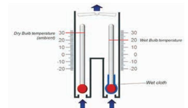
Figure 1: Wet bulb and dry bulb temperatures
