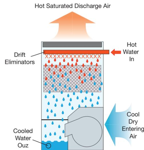
Figure 8: Forced draft cooling tower
